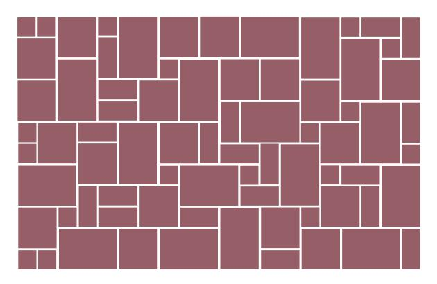
Lay a suitable sub base material such as a crushed hardcore well compacted onto the subgrade. This is followed by a 30-50mm laying course of concrete made up of 6 parts sharp sand and 1 part cement.
